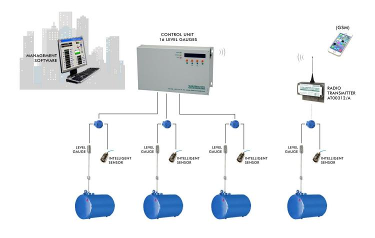
Level measurement and leakage alarm monitoring control unit for tanks, piping and wells. Management of 16 level guages and 32 leakage alarm sensors, 4/8 on/off inputs and up to 8 relays with programmable-event outputs. It can be connected to other 4 devices to extend the level, alarm and relay control and to allow interfacing with main control systems installed on refuelling stations.
